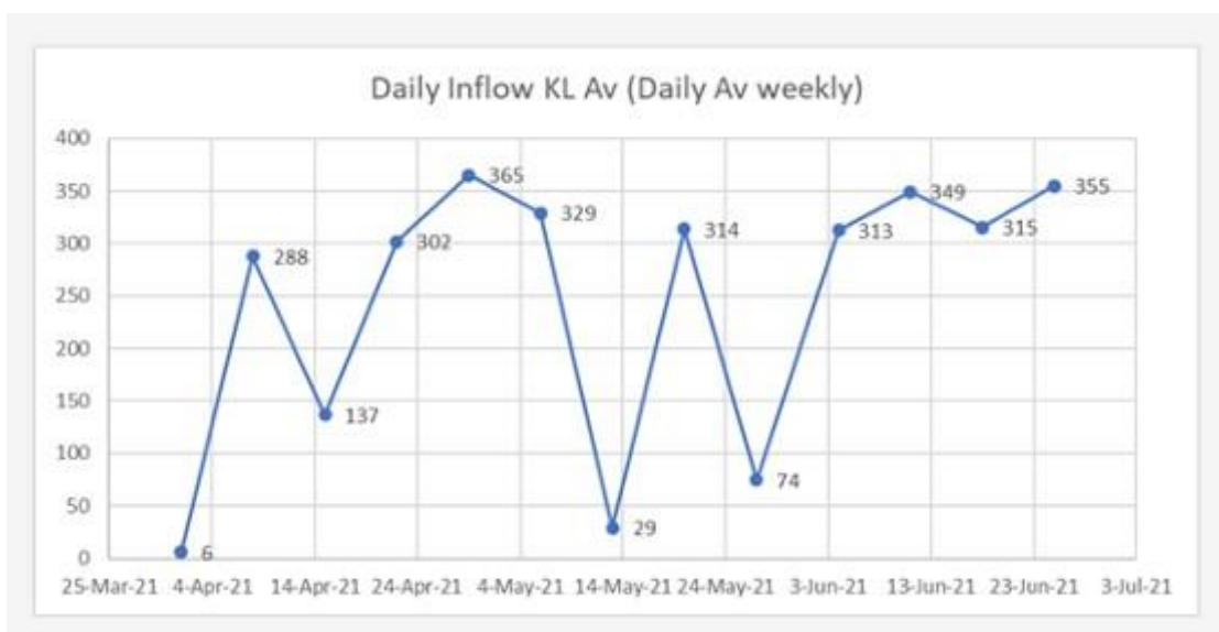
Average daily wastewater volumes received from BHP ODS Camp between 1 April and 30 June 2021.
