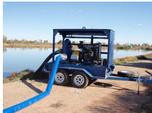
New pump trailer enables us to move water around the sewer lagoons much quicker, a saving of 65% on man hours
