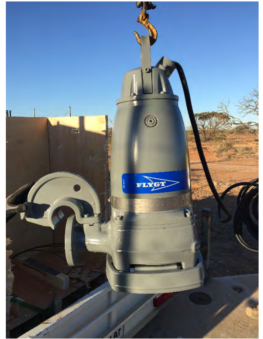
Chopper type pump installed at Pump Station H to reduce ongoing blockage issues
